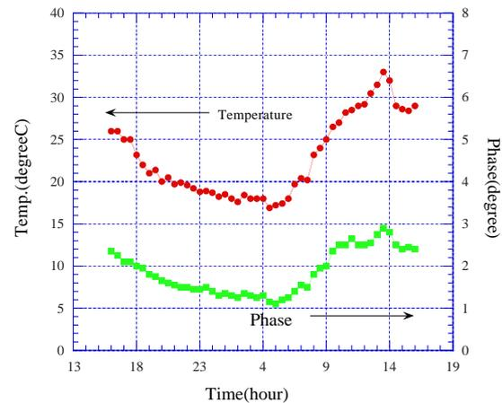
Fig. 3 Phase stability of the reference signal(508MHz) distribution system - Two LCRs have a 500m long cable distance, the phase change is less than 2°(10ps) with 15°C temperature change .
