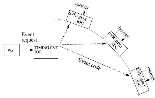
Fig.2 Configuration of the synchronization of the BPM data acquisition.
