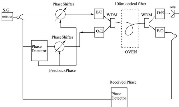
Fig. 4 Measurement set up of the PLL feedback using the optical link.
