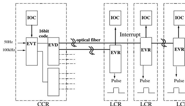
Fig.1 Layout of the Software trigger system - an EVT(event transmitter module) produces 16 bit codes, EVDs(event distribution modules) distribute the codes using the multi-mode optical link, and EVRs(event receiver modules) decode the code. If the sent data matches with the preset data then it generates a synchronized pulse or interrupt to each IOC.
