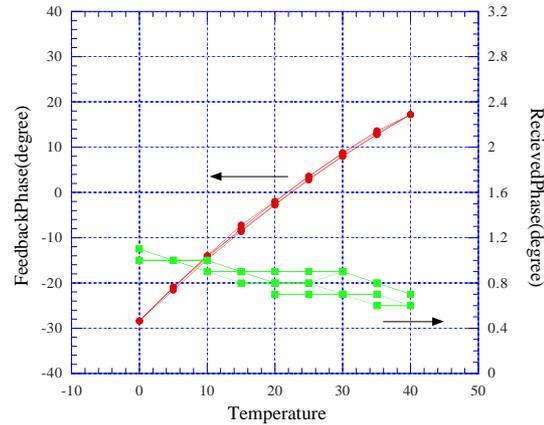
Fig. 5 Measurement of the feedback phase and the received phase
