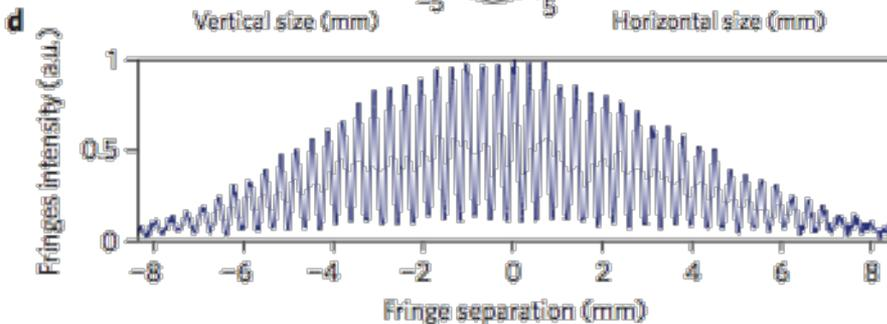
The **transverse spatial mode** has been measured to be very close to the **TEM00** mode and also coherence measurements indicate a very **high degree of transverse coherence**.
