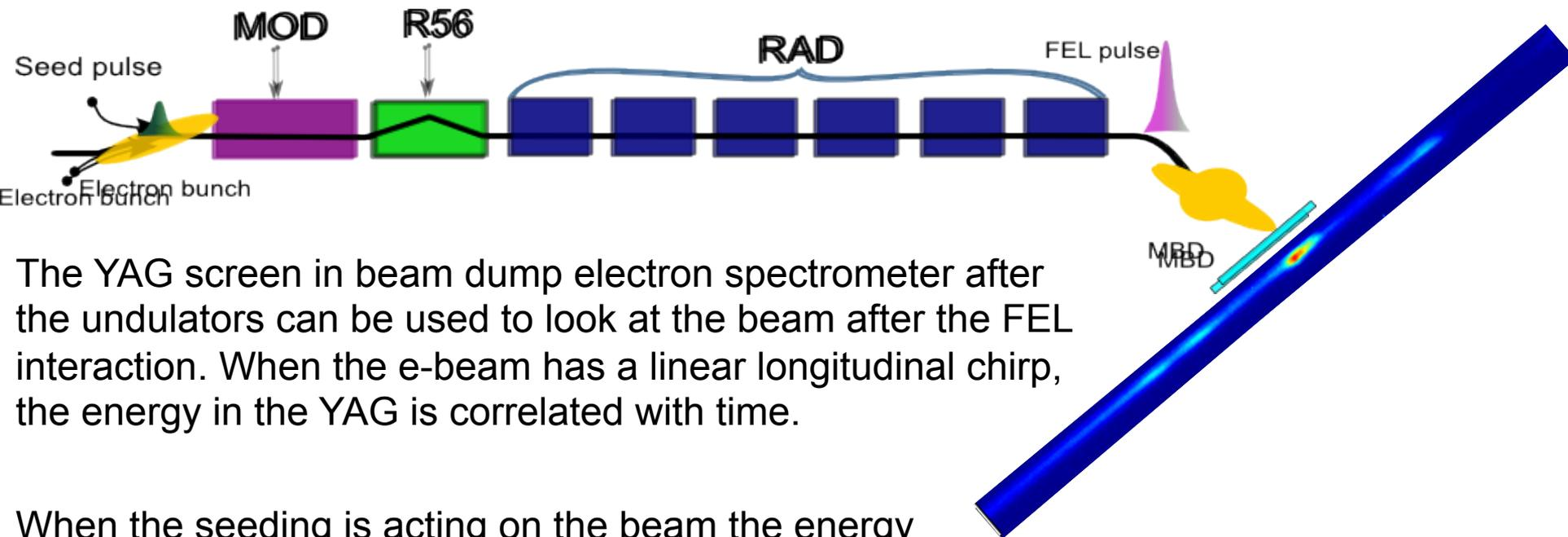
The YAG screen in beam dump electron spectrometer after the undulators can be used to look at the beam after the FEL interaction. When the e-beam has a linear longitudinal chirp, the energy in the YAG is correlated with time.
