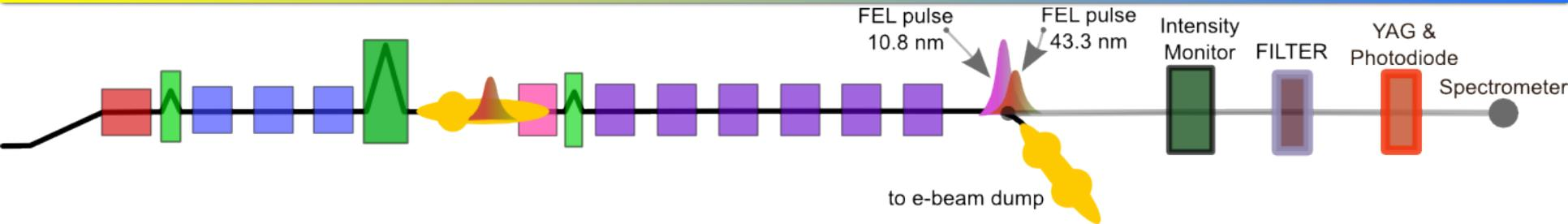
Optimized the electron beam and aligned the FEL and diagnostic looking at the first stage radiation at 43 nm.
