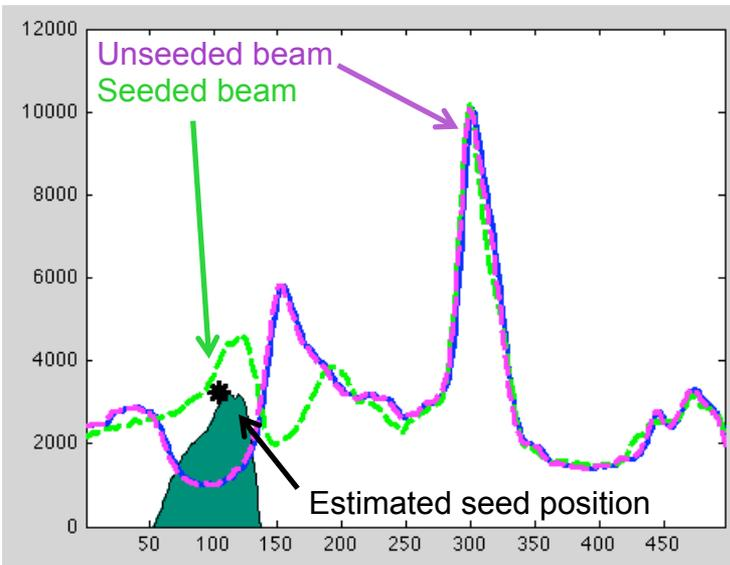
From a sequence of spectra we can follow the evolution of e-beam – laser timing.
