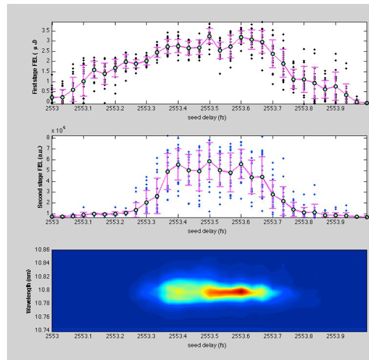
Using the FEL diagnostic we can measure at the same time the radiation produced by the first stage at 43 nm and the one produced by the second stage 10.8nm.
