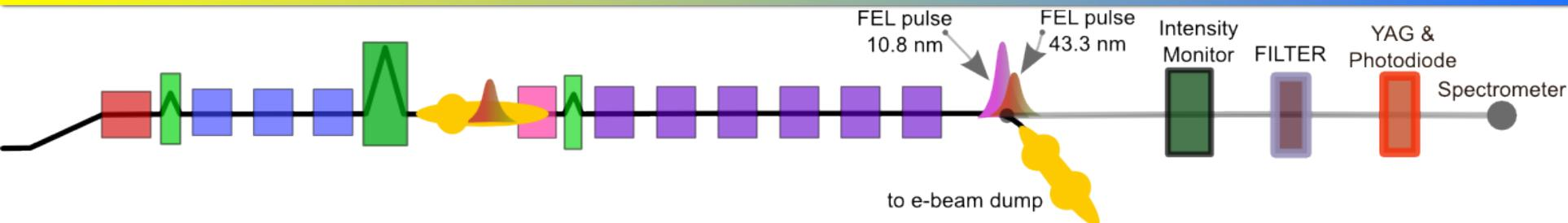
Using intensity monitor and the photodiode after the filter it is possible to measure simultaneously the power from the first and the second stage.
