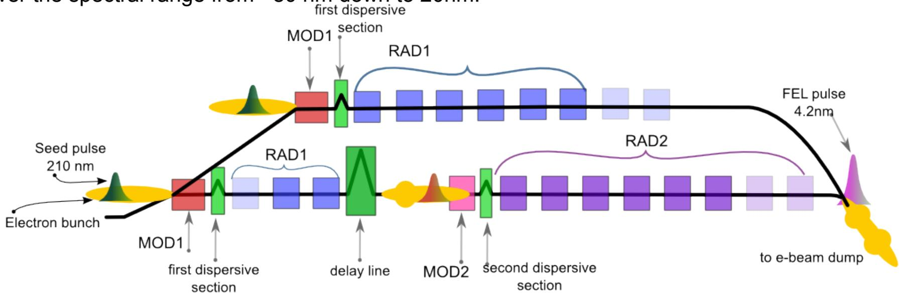
FEL-2, in order to be able to reach the wavelength range from 20 to ~4 nm starting from a seed laser in the UV, is based on a double cascade of high gain harmonic generation. The nominal layout uses a magnetic electron delay line in order to improve the FEL performance by using the fresh bunch technique. Other FEL configurations are also possible in the future (e.g. EEHG).
