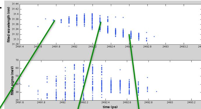
When the seeding is placed on the minimum of the of the electron beam energy the tail and the head of the seed see a different electron beam chirp and the FEL spectrum is splitted.
