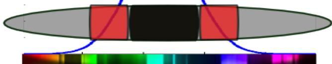
Seeding with a **chirped laser** allows to produce two **FEL pulses separated in time and spectrum**. Time and frequency separation can be controlled acting on the seed laser and on FEL parameters\*\*.
