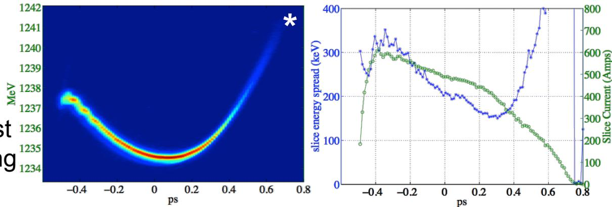
By properly tuning the X-band and the RF phase of the last part of the linac it is possible to mitigate the effect of wakefield and reduce the quadratic chirp.
