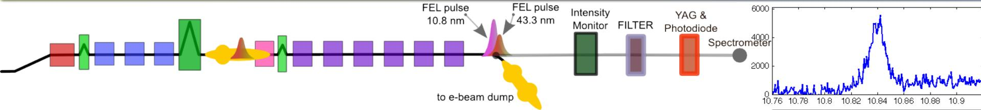
The exponential growth of the power on the second radiator has been measured both looking at a YAG after a filter that stops the first stage radiation and at the spectrum intensity.
