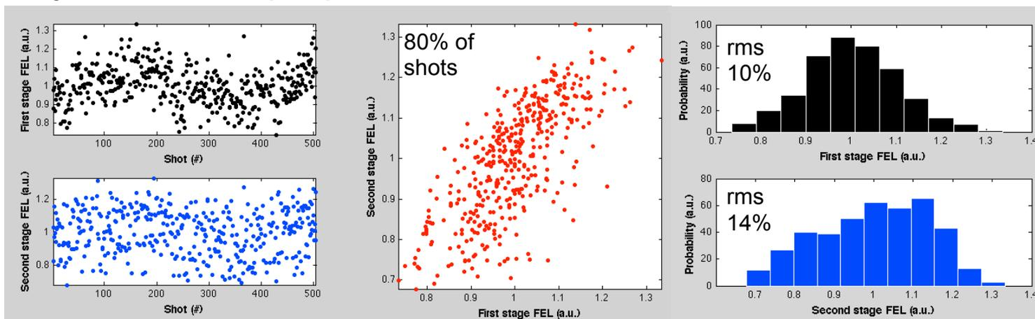
These data refer to the case of 260 → 43 → 10.8 nm. In this configuration the power from the first stage is more than enough for seeding and it is generally needed to keep it down to maximize the power from the second stage.
