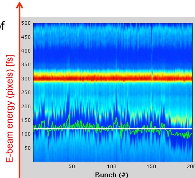
A procedure has been implemented to detect the position of the seed laser from the difference between seeded and unseeded e-beam spectra
