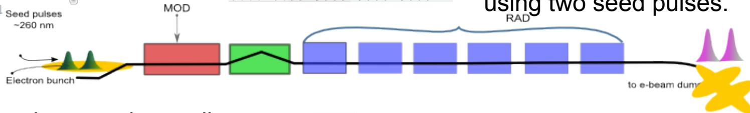
Delay between two pulses can be easily controlled and also the two wavelengths can be slightly different.
