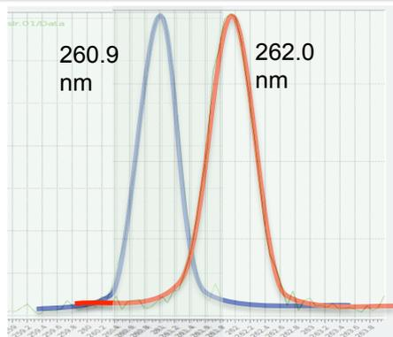
In order to allow a wider temporal separation between the two pulses required by one of the FERMI users we also implemented a scheme using two seed pulses.
