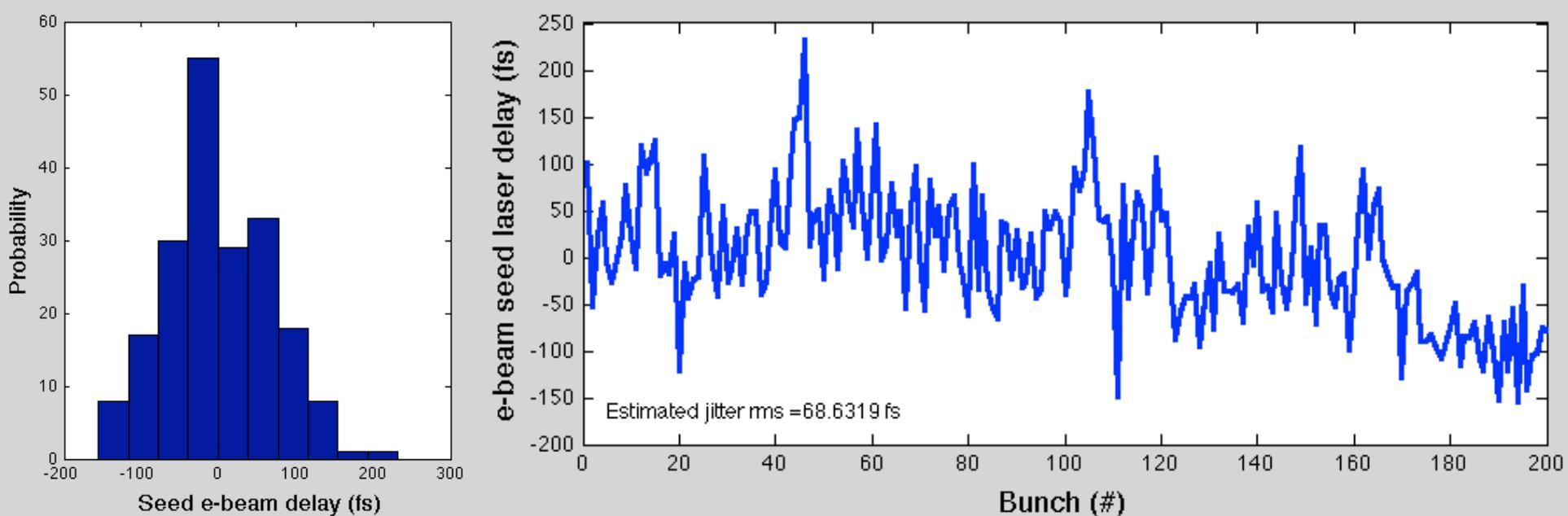
In RUN13 an optical locking system of the seed laser has been installed. The obtained improvement in the FEL stability suggests a reduced timing jitter that has not yet been measured with such a technique.
