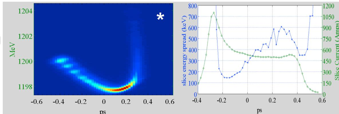
FEL process is initiated by the seed laser interacting with the electron beam. The timing between the two is critical for having a stable FEL.
