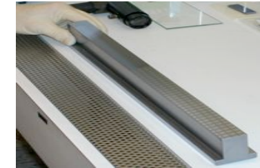
Coating of Synchrotron Mirror up to 150 cm
