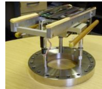
The optic mount used to hold and manoeuvre the optic within the X-ray tunnel test facility
