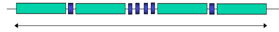
Fig. 3 A sketch of 25 meter-long achromatic cell for 10 and 20 GeV arcs in the eRHIC's ERL.
