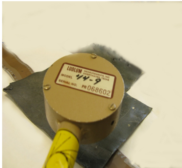
Fig.3 - Exposed film with sheet of lead containing a pin-hole (not visible) and the Ludlum Model 12 survey meter equipped with a pancake probe to ascertain the area on the film with the maximum activation. Once maximum activation had been located, the film was transferred back to its original exposure placement and the loss point transferred from the film to the beam pipe to determine where beam was being lost.
