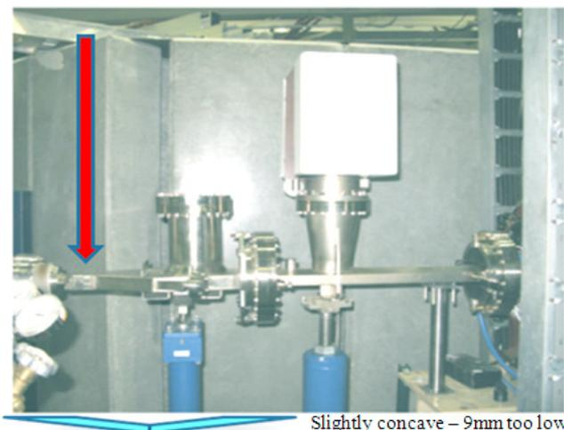
*Fig.5 - Location of radiation source as a consequence of the beam-pipe being 9 mm too low. Point was identified by unique method of using exposed photographic film and looking for activation of  $^{107}\text{Ag}$  to  $^{108}\text{Ag}$  in the film emulsion. This isotope has a  $T_{1/2}$  of 2.39 minutes. BMP's had been unable to detect this anomaly. With the beam pipe in the correct position, radiation dose was reduced from 72mSv to 32 $\mu$ Sv.*
