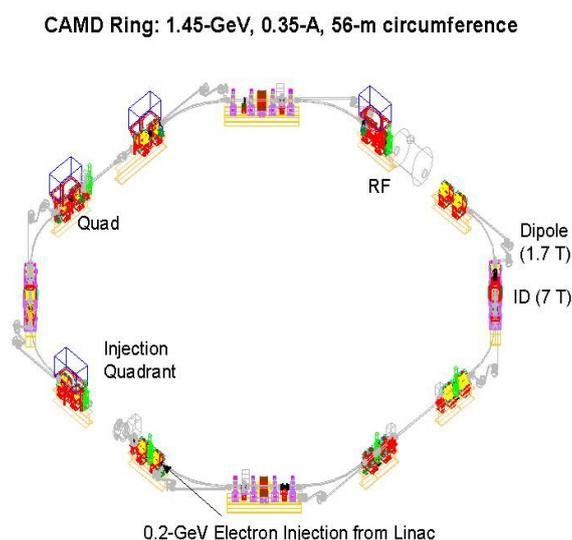
Fig.1 - Layout of the CAMD Storage ring.
