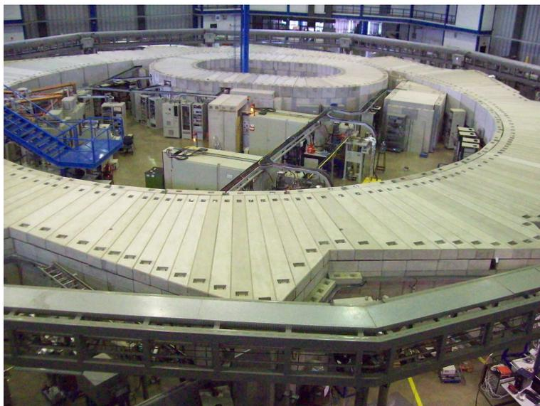
*Fig.3 - Current operation type of the LNLS light source: it was constructed a Booster and installed concrete roof and inner wall. After that and other improvements people were allowed to stay at experimental hall during injections.*
