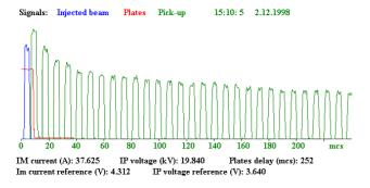
Figure 3: Example of the bunch intensity and shape measurement during first turns (RF off).
