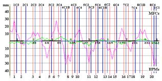
Figure 4: X-closed orbit before and after correction.
