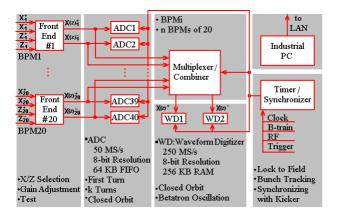
Figure 5: Structural model of BPM hardware.
