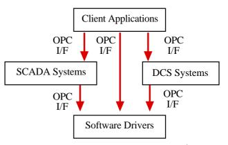
Figure 1: Example of where OPC may be applied<sup>1</sup>.
