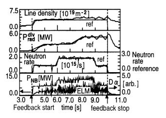
Figure 5 Demonstration of the simultaneous feedback control of 3 kinetic parameters on JT-60U tokamak: line density, radiated power fraction in the divertor region and the neutron production rate. The feedback of the Neutral Beam injection power is shown chopped according to the feedback control signal.
