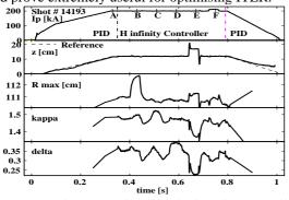
Figure 3 Switching in and out the high-order controller to replace the PID controller. The pulses on the controlled parameters are used to test the closed-loop response.
