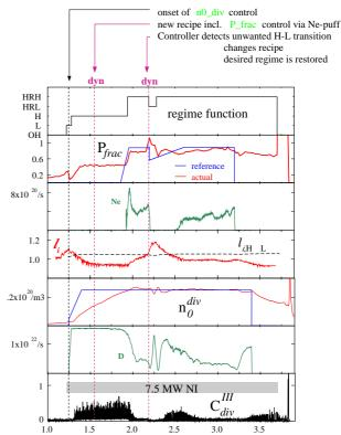
Figure 4 Plasma regime classification as a function of time. The controller switches the Pfrac radiated power fraction demand signal to force the desired mode to be recovered. The reference returns to its original value once the H-mode is recovered.
