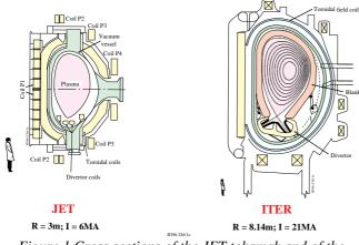
. Figure 1 Cross sections of the JET tokamak and of the ITER reactor design
