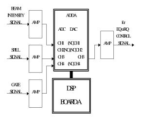
Figure 2: The test circuit of digital feedback
