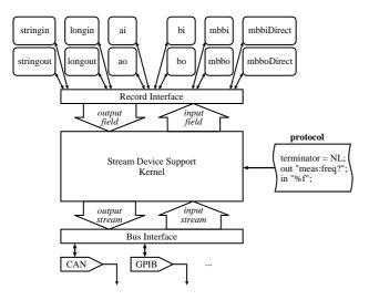
Figure 2: Interactions of the Stream Device Support [7].
