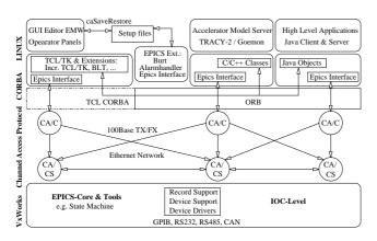
Figure 1: Layout of the Control Software Layers.
