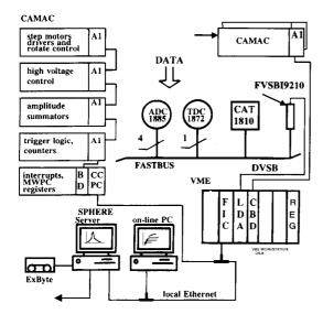
Figure 2: Architecture of the data acquisition system.
