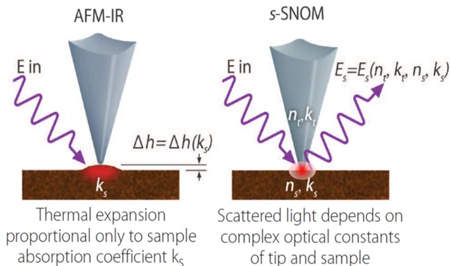
Figure: Close-up view of the laser light/AFM tip/sample interaction for the AFM-IR (left) and s-SNOM (right) experiments.
