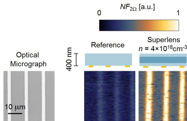
Fig. 1: Near-field image (second harmonic demodulation) of  $2\ \mu\text{m}$  thick gold stripes using a superlens and a reference sample (400 nm thick intrinsic GaAs). Both images were obtained at 15 THz, the resonance frequency of the superlens. On the left, an optical image of the gold stripes is depicted.
