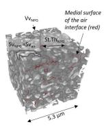
of the network structure with deformation. X-ray Tomographic Microscopy (XTM) on the other hand allows for *in situ* observation of the 3D nanostructural evolution during mechanical testing. Since gold is high absorbing for X-rays, NPG is also an optimal sample for evaluating the capability of an XTM setup.
