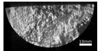
Fig. 1. Example of the CT reconstruction of the Galena mineral (lead-sulfide in the quarth matrix) with mean density of  $8.3g/cm^3$  (73% of the pure lead).
