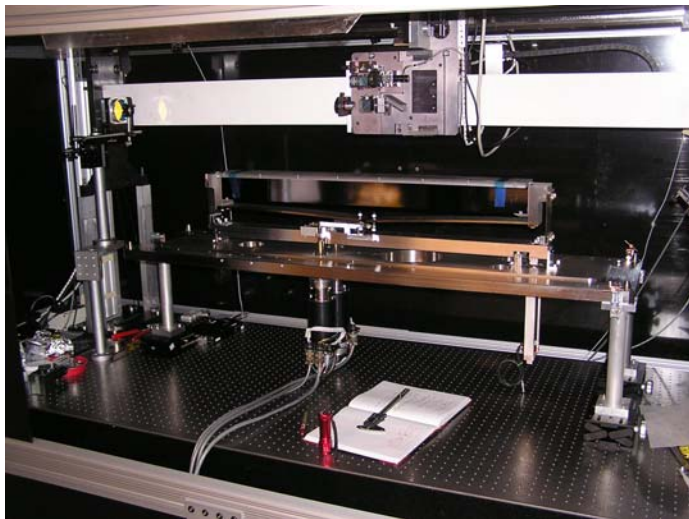
Figure 1: An example of a bendable optic used at ALS beamline 5.0.2. The mirror with a 900mm long substrate is shown on the Long Trace Profiler (LTP) optical table to be adjusted to the desired spherical shape with radius of curvature of about 2300 m.
