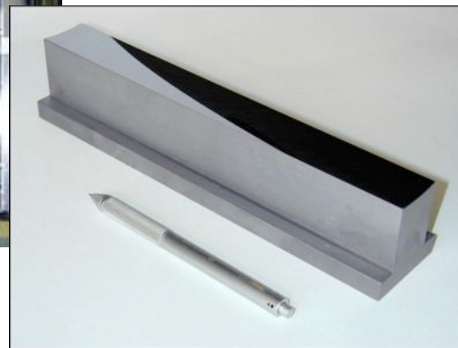
Toroidal mirror for synchrotron
