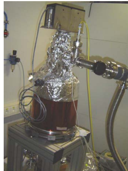
Setting high vacuum 2.10^{-8}\text{mbar} 6 days – baking up to 120^\circ \text{C}
