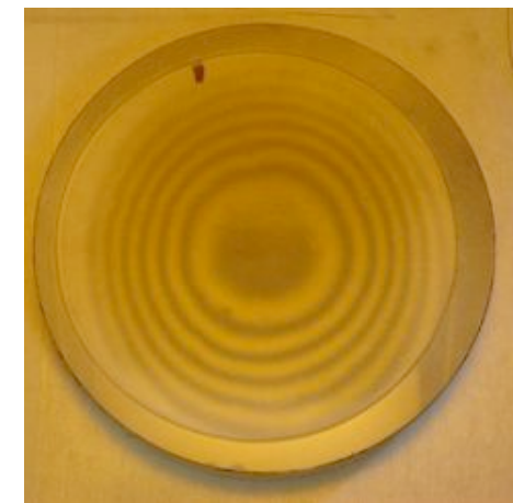
Fringes between mould and glass: very circular and without dust contamination
