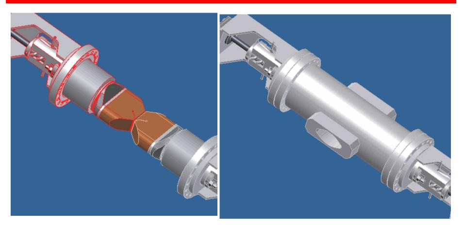
Thickness in beam direction ~75mm Cu (~5.25 X) Average Beam Energy Loss ~99.5%, Required Local Shielding to Reduce Dose Rates Outside the Shield Wall
