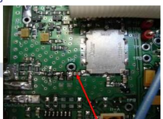
serial capacitor cracked
