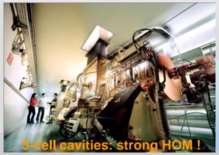
$R/Q = 139 \ \Omega / cell$  Qo = 38500  $Rs = 26.8 \ M\Omega \ (5 \ cells)$   $V_{nom} = 1.4 \ ... \ 2.5 \ MV$   $2 \ couplers: \ \beta_{max} = 4.4$  $Max \ 170 \ kW \ / \ coupler$
