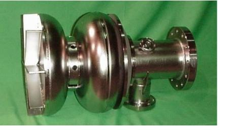
1.5 cell SRF photo injector cavity produced by CEBAF in cooperation with HZB, DESY and the Soltan Institute (Poland).
