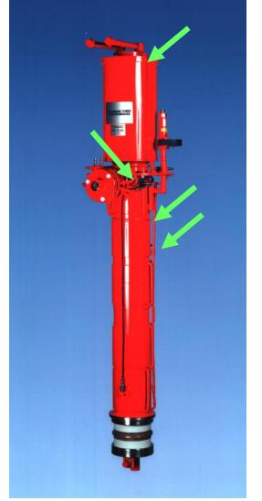
water leaks on new Thales klystron
