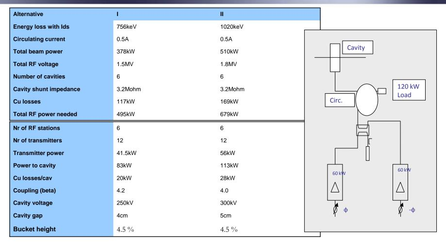
Alt I: Represents a solution for a 60% ID equipped ring, with the present MAX II/ MAX III cavities.
