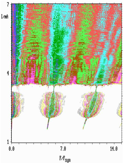
BBR: R<sub>s</sub>=10 kΩ, F<sub>res</sub>=40 GHz, Q=1 R= 850 Ω and L/ $\omega_0$ =0.2 Ω
