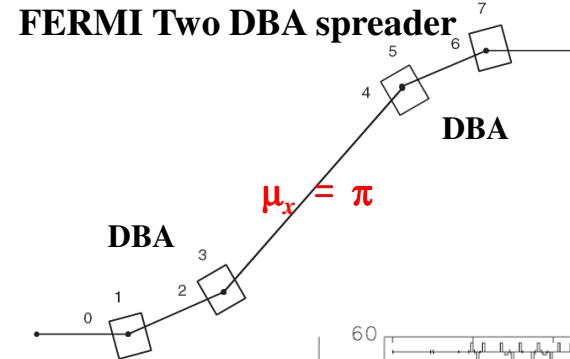
When the phase advance between two DBAs is  $\pi$ , the CSR induced emittance growth can be minimized.
