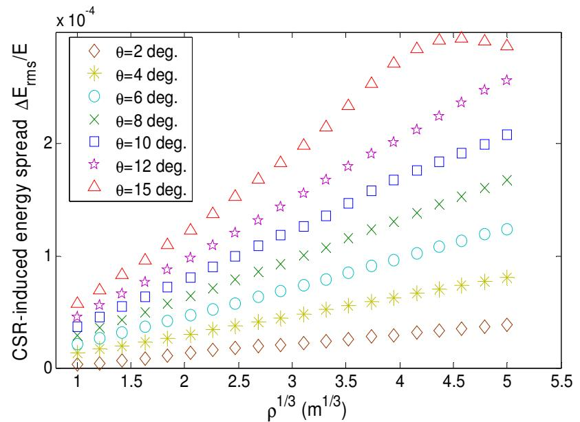
This linear relation applies well to the cases with  $\theta$  from 1 to 12 degrees and  $\rho$  from 1 to 150 m.
