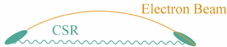
(1) CSR emission from the bunch tail catches up with the bunch head
