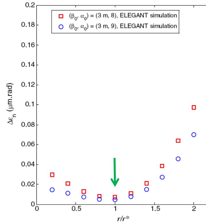
$$\Delta\epsilon_n \Big|_{r=r^*} \approx \frac{1}{2} \gamma \beta k_{rms}^2 S_1^2 (\theta_1 + r^{*1/3} \theta_2)^2 \rho_1^{2/3} \beta_1 [1 - M_{c2c}(2,1) / M_{c2c}^*(2,1)]^2. \quad r \equiv \rho_2 / \rho_1, \text{ and } r^* = 27/8 \text{ in this case}$$
